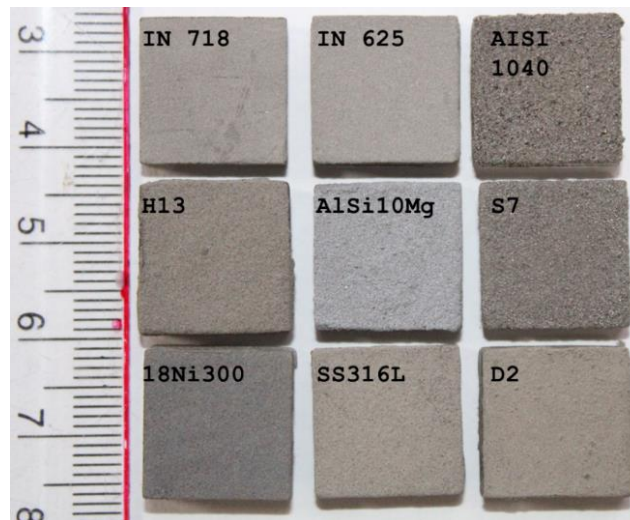
Fig. 2.9: Metal powders that are considered subjects for the calculation of COSF against the SS316L test platform
