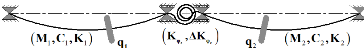
Figure 3-2 Coupled simple rotor system with displacements at disc locations
