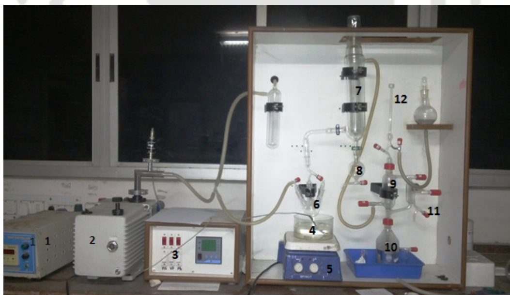
1. PID Controller; 2. Vacuum pump; 3. Pirani gauge; 4. Oil bath; 5. Heater; 6. Reactor; 7. Condenser; 8. Collector flask; 9. Gas Chamber; 10. Mercury vessel; 11. Air valve; 12. Gas burette
