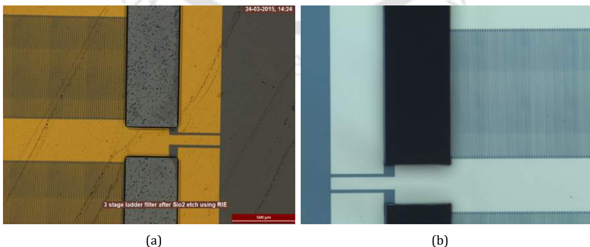
Fig. 7.9. (a) Microscopic image of ER device after RIE process (b) ER type device after DRIE process showing the vertically developed groove.
