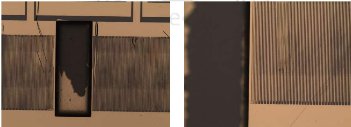
Fig. 7.6. Microscopic images of developed IDT structure after the development of micromachined grooves.
