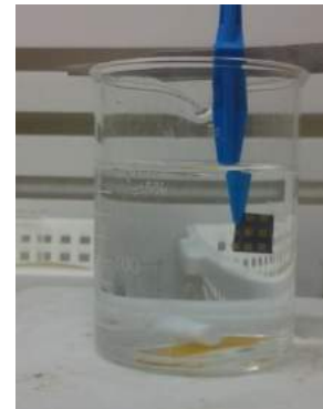
Fig. 4.9. (a) Illustration of conventional flow of etchant over the device, the cross-section along the aperture is depicted and (b) experimental setup for patterning of ZnO film using magnetic stirrer.
