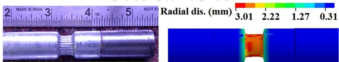
Fig. 3.10 Final shapes obtained in (a) experiment and (b) simulation
