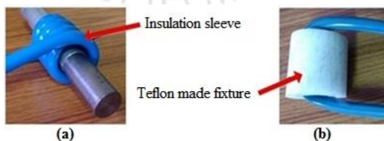
Fig. 4. 2 (a) Experimental setup and (b) coil inside Teflon made a fixture
