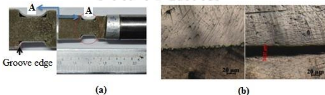
Fig. 3.26 (a) Cross-sectional view of joining zone and (b) metallographic image at the joining zone
