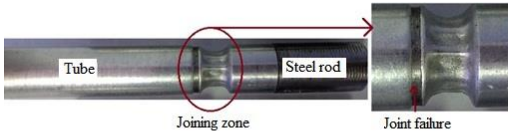
Fig. 3.22 Crimped sample after the pull-out test
