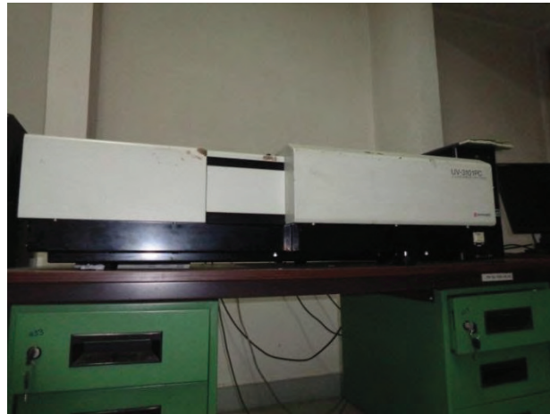
Figure 2.4: Experimental setup of UV-Vis-NIR spectroscopy.
