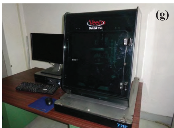
Figure 2.3: Experimental setup of different characterization techniques: (a) Field emission scanning electron microscopy, (b) Atomic force microscopy, (c) X-ray diffraction, (d) Raman spectroscopy, (e) Fourier transform infrared spectroscopy, (f) transmission electron microscopy and (g) Stylus profilometer.
