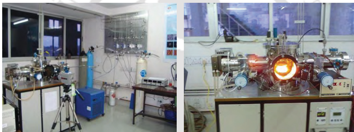
Figure 2.2: Designed HFCVD system with gas manifold in our laboratory (left) and HFCVD system during deposition of the films (right).
