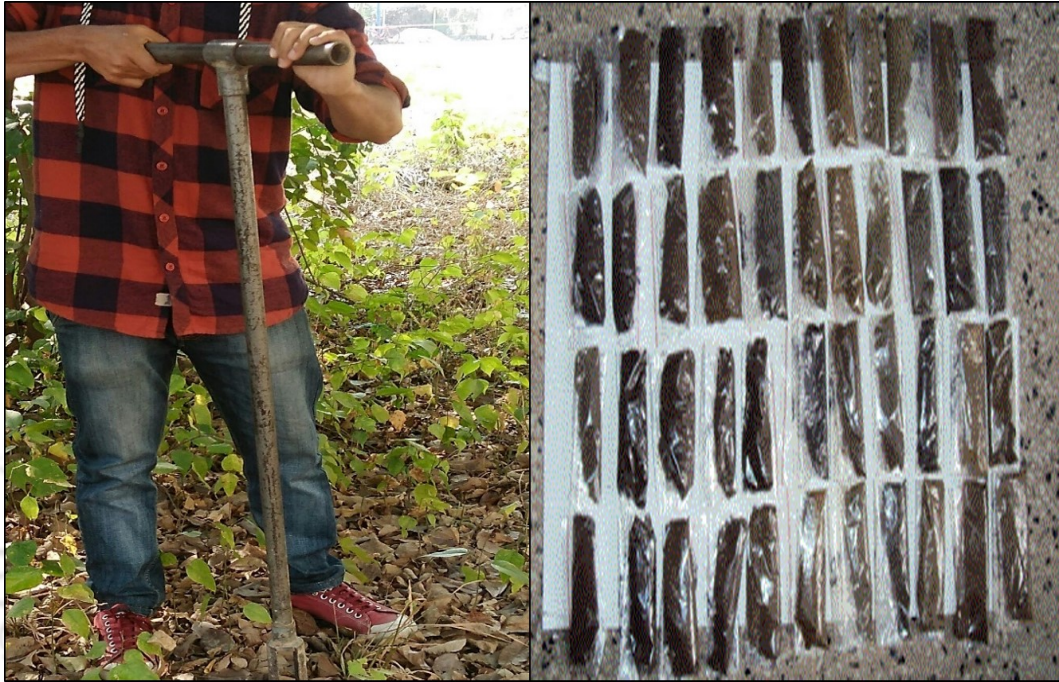
Figure 2.2: Soil samples collection using core cutter (left) and soil samples preparation (right)
