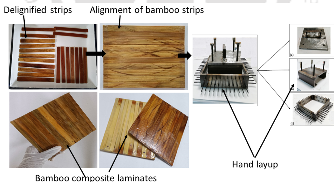
Figure 3.3: Developed bamboo-epoxy composite laminates.
