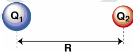
Figure 1.5: Ionic interactions between two atoms Q_1 and Q_2 at a distance R .
