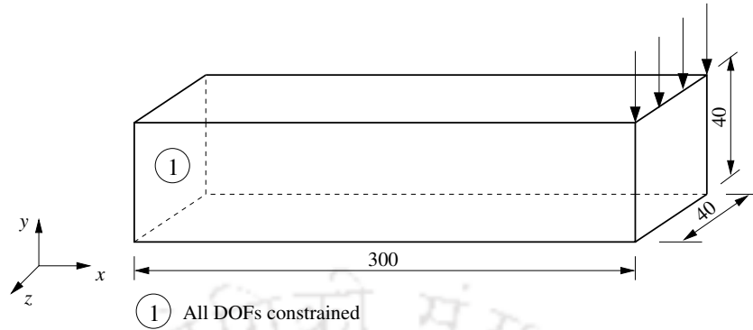
Figure 5.17: A cantilever beam with end load. All dimensions are taken in millimeters (mm).
