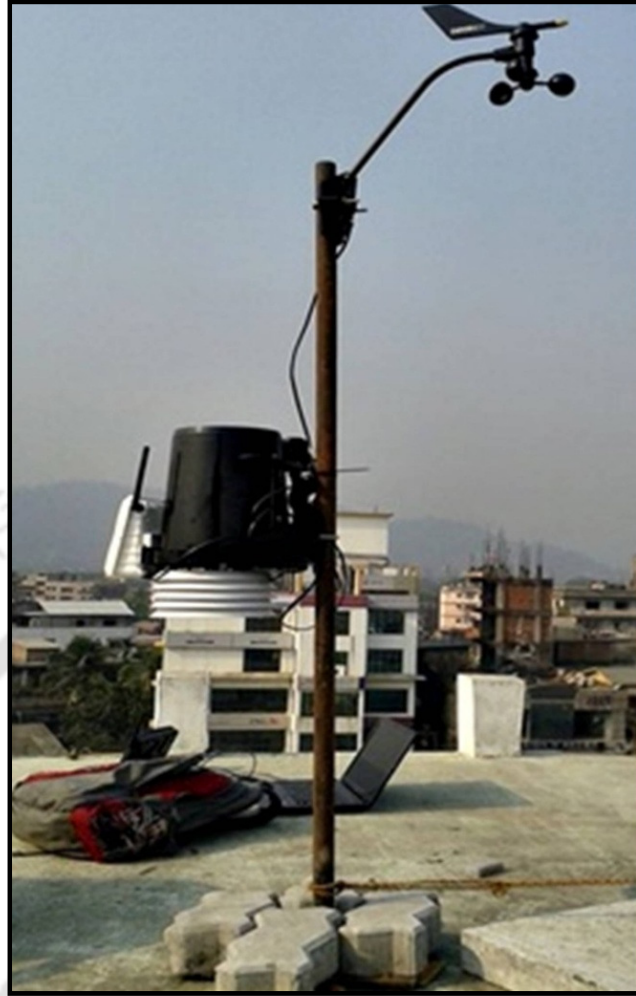
Figure 3.3: Picture shows the meteorological monitoring instrument (Wireless Vantage Pro2, model no: 6152) at the installed location
