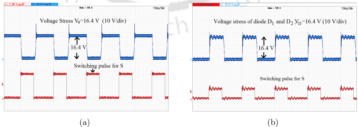
Figure 5.17: Experimental result of voltage stresses (a) v_S , and (b) v_D for \alpha = 0.40
