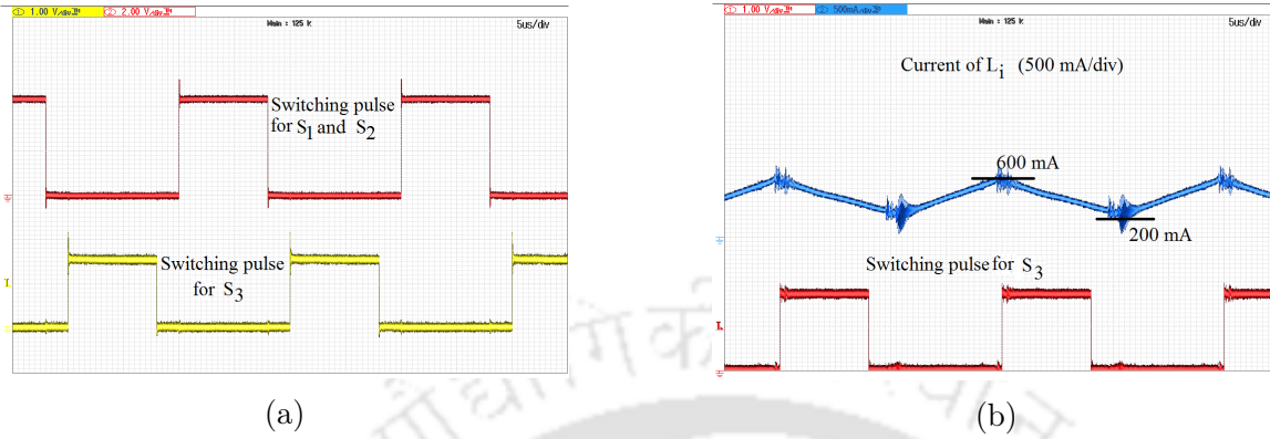
Figure 3.17: Experimental waveform for \alpha = 0.40 (a) Two-phase switching pulses, and (b) i_{L_i}
