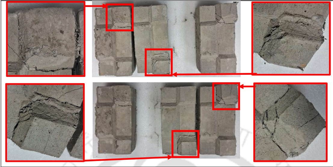
Figure 6.8: (C) Typical failure pattern of FCIB prisms (triplets) under shear forces perpendicular to header face.
