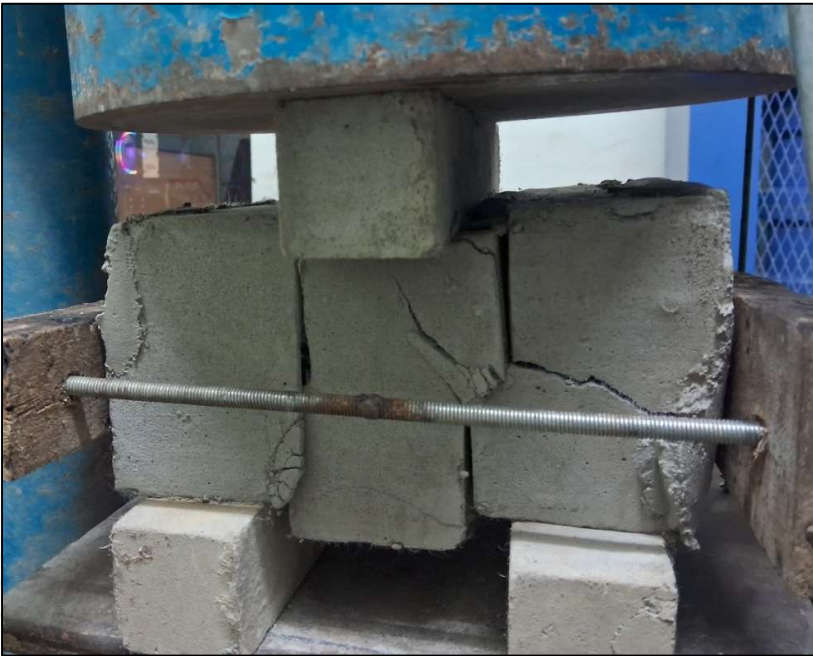
Figure 6.7: (B) Typical loading setup for testing shear resistance (perpendicular to stretcher face) between FCIB triplets.
