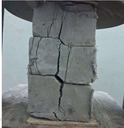
Figure 6.6: (C) Typical failure pattern (header face) of FCIB prisms (triplets) under compression.
