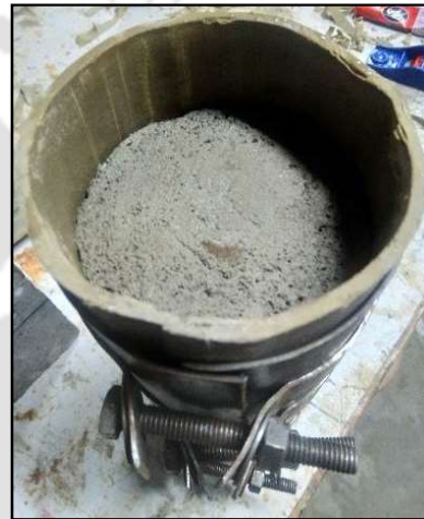
Figure 4.1: (B) Setup with rubber tube and iron clamp for sealing the sample.
