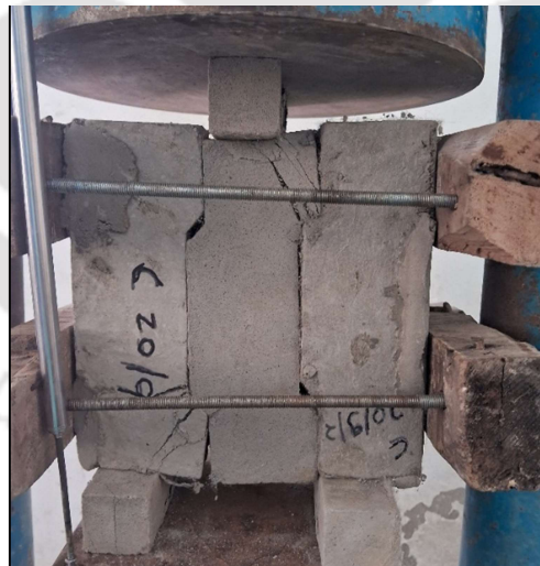
Figure 6.7: (A) Typical loading setup for testing shear resistance (perpendicular to header face) between FCIB triplets.
