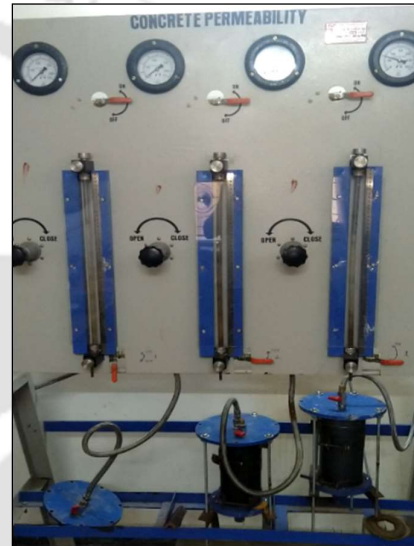
Figure 4.2: (B) Experimental setup to measure concrete permeability.
