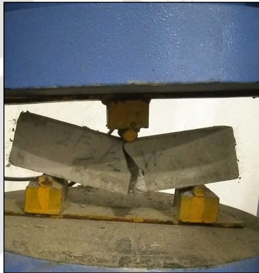
Figure 5.20: (B) Post failure behaviour of FC2 mixes with PP fiber during flexural strength test.
