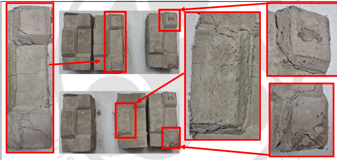
Figure 6.8: (D) Typical failure pattern of FCIB prisms (triplets) under shear forces perpendicular to stretcher face.
