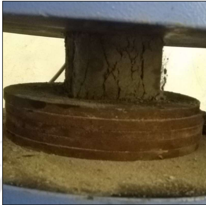
Figure 6.4: (C) Typical failure pattern of FC cube of 50 mm dimension under compression.
