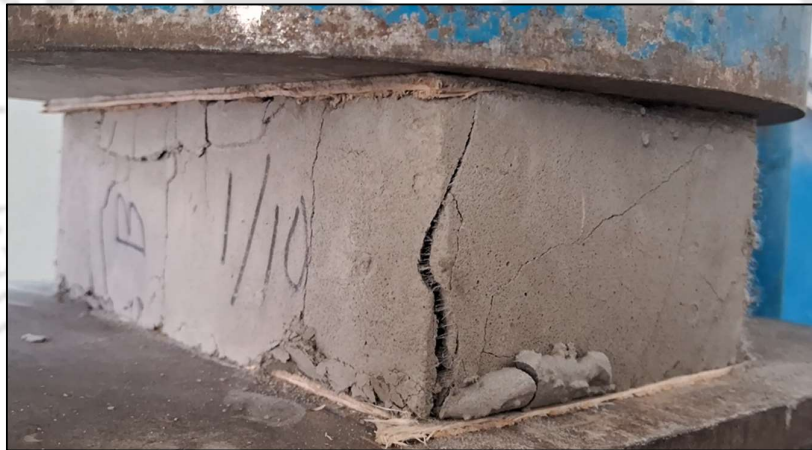
Figure 6.4: (B) Typical failure pattern of FCIB under compression.
