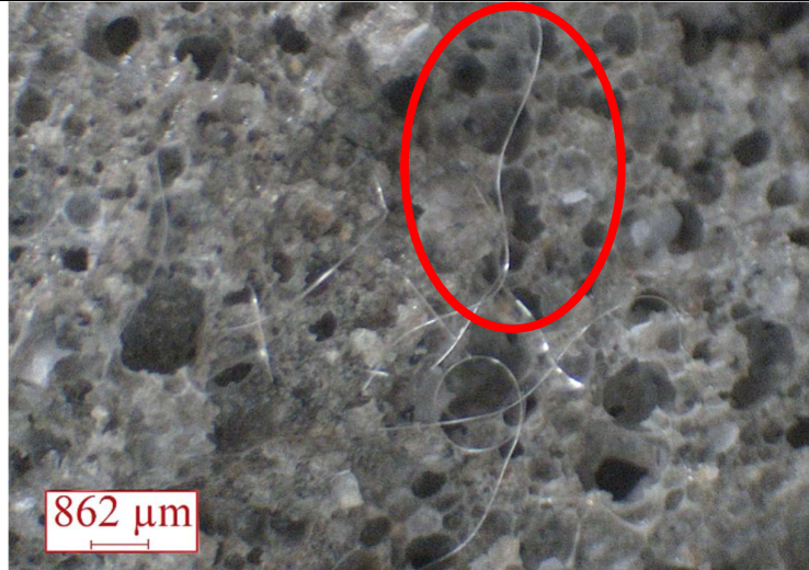
Figure 4.11: (B) Optical microscopic image of FC1Ps mix at 0.7X depicting pore connectivity.
