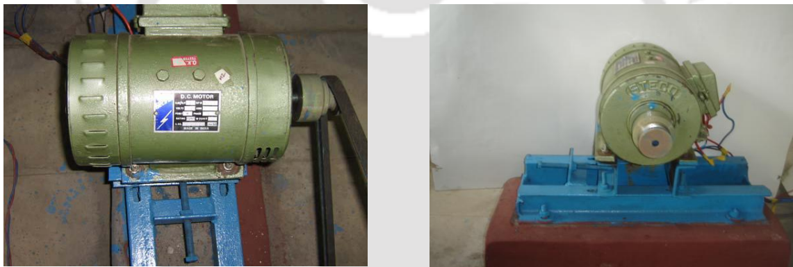
Figure C.2: DC motor arrangement with channel framework
