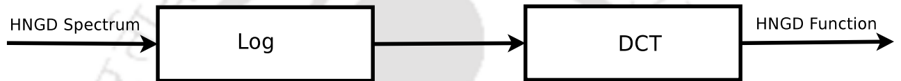
Figure 5.5: Block diagram showing the steps of conversion of HNGD spectra to the HNGD function (HNGDF) feature
