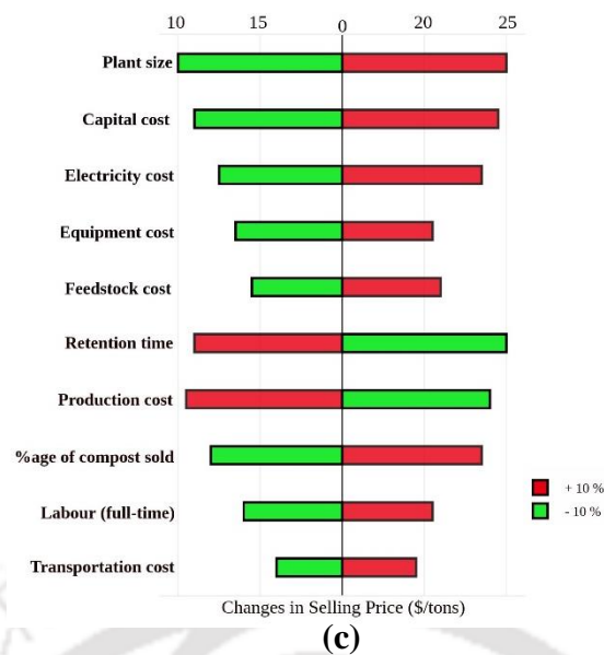
Fig. 10.6 Sensitivity analysis of the composting process profitability for (a) HSCF (b) MSCF and (c) YWCF systems
