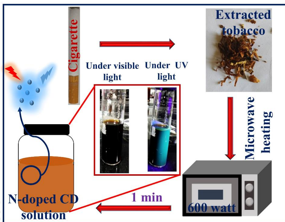
Scheme 3.1. Schematic representation of the synthesis steps of the CDs. The photographs of the CD solution in the presence and absence of UV light are shown in the inset.
