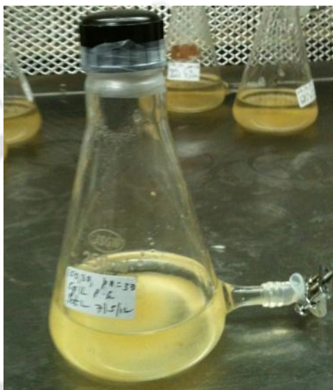
Figure A1 Picture of a custom fabricated Erlenmeyer flasks for anaerobic fermentation
