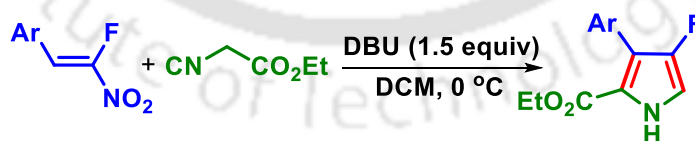
Scheme I.2. Barton-Zard reaction of \beta -nitrostyrene with isocyanoacetate.
