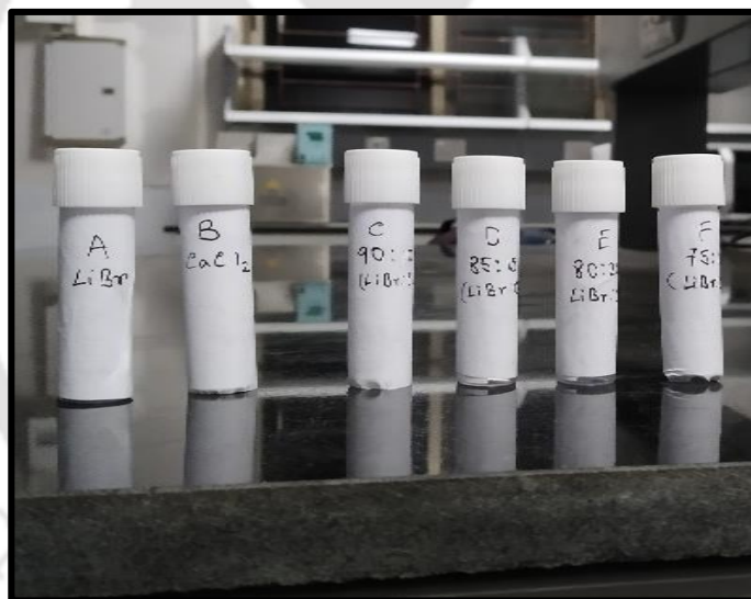
Fig. 3.11: Image of prepared samples ( a: LiBr; b: \text{CaCl}_2 ; c-f: LiBr: \text{CaCl}_2 (c: 90:10; d: 85:15; e: 80:20 and f: 75:25))
