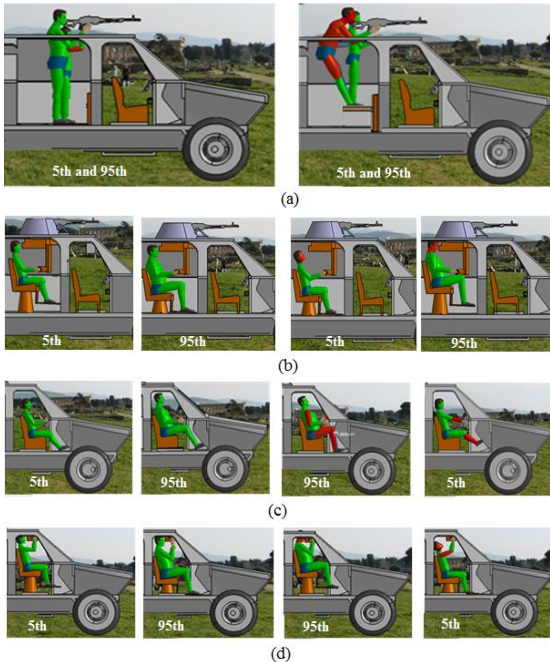
Figure 5. 4: Comfort/discomfort analyses of a) gunners in standing posture with 5 th p female and 95 th p male manikins b) gunners in sitting posture with 5 th p female and 95 th p male manikins c) driver with 5 th p female and 95 th p male manikin d) driver with 5 th p female and 95 th manikin.
