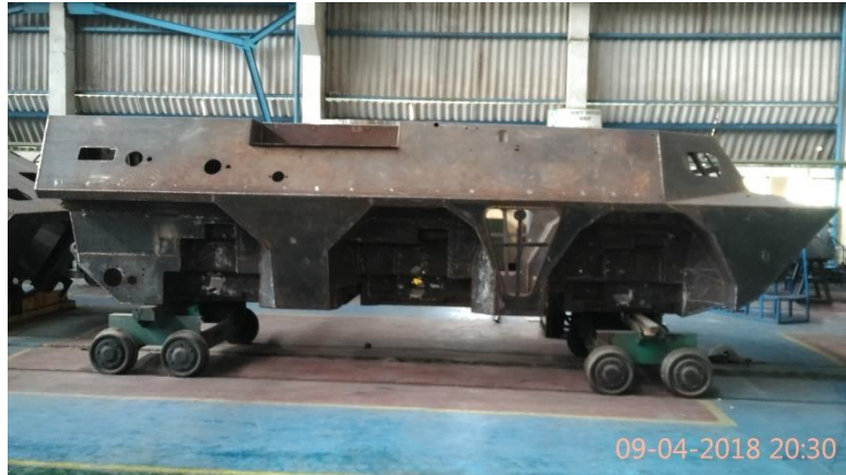
Figure 4. 8: Hull structure of existing Ethiopian armoured vehicle called APC (Photo taken from Bisoftu Automotive and Locomotive Industry, Ethiopia)
