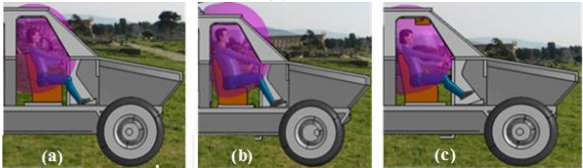
Figure 5. 5: Reachability analysis of the driver workspace of DMU (a) with 5 th p female manikin at forward-most position (b) with 95 th p male manikin at rearward most position (c) with 5 th p female manikin at rearward most position
