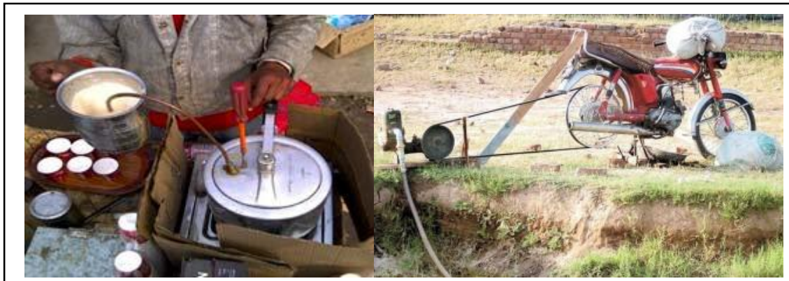
Figure 2.13: Examples of Jugaad, Coffee making with pressure cooker and pumping water by bike
