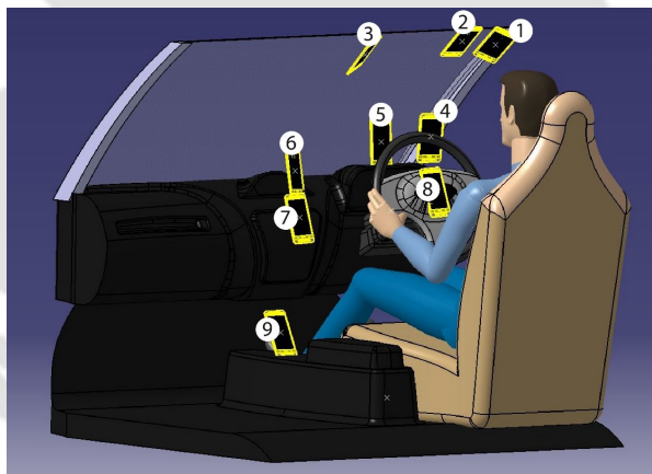
Figure 4.4: Isometric view of nine different mobile positions around the steering wheel and dashboard
