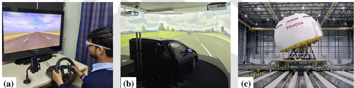
Figure 2.4: A typical classification of driving simulators (a) low-level fidelity, (b) mid-level fidelity, and (c) high-level fidelity
