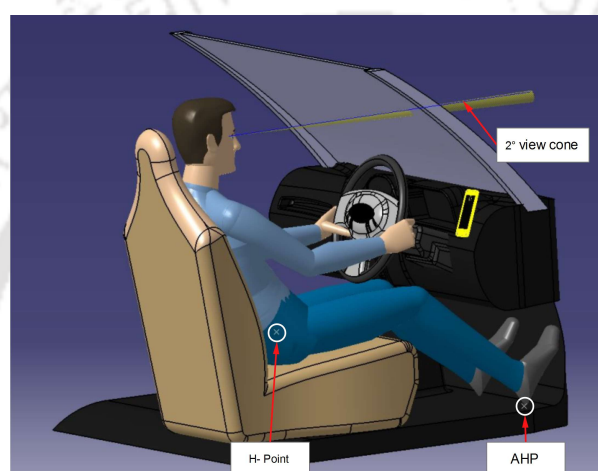
Figure 4.5: Digital human model (manikin) interfaced with a virtual car dashboard with reference points
