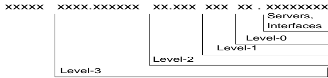
FIGURE 6.3: Encoding DCell address in an IP address
