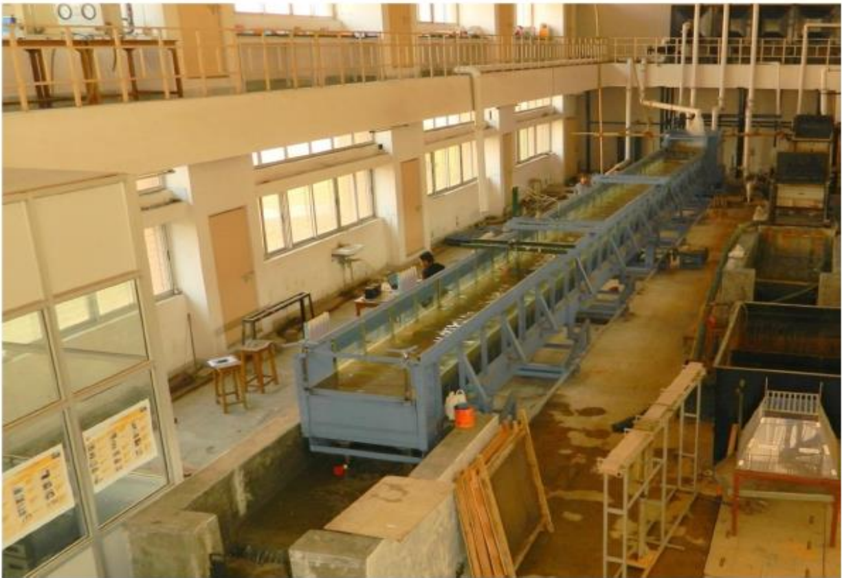
Figure 2.2 Photograph of the tilting flume
