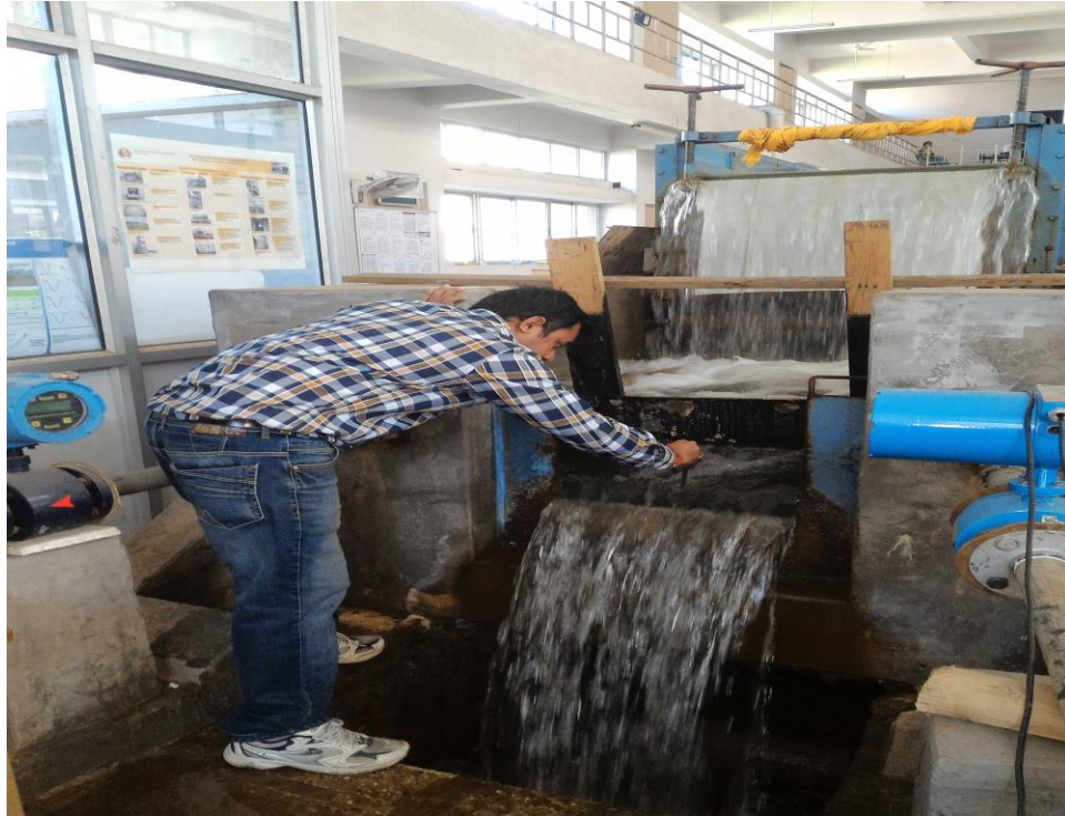
Figure 2.6: Measurement of flow discharge in the main channel discharge
