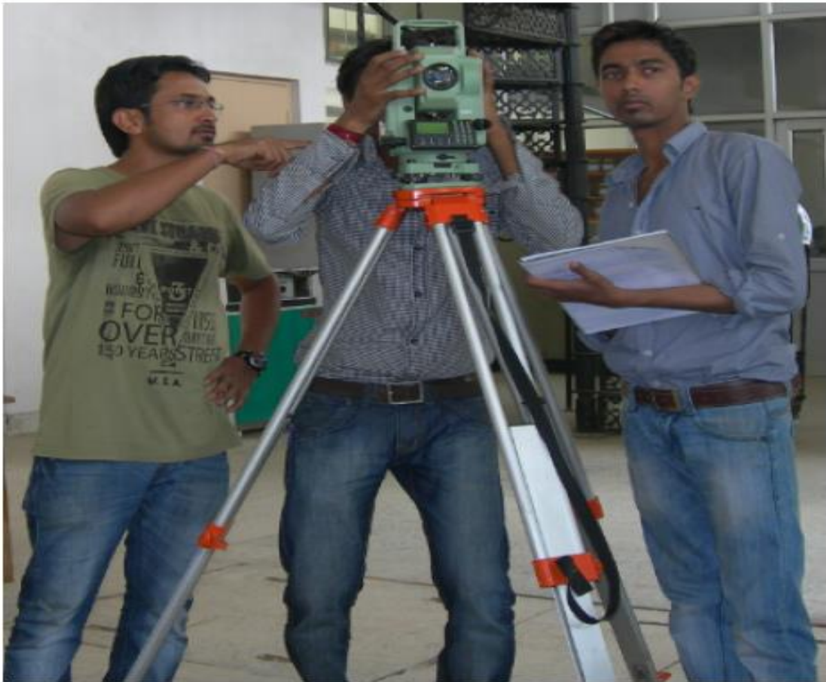
Figure 2.11: Total station for measuring bed slope
