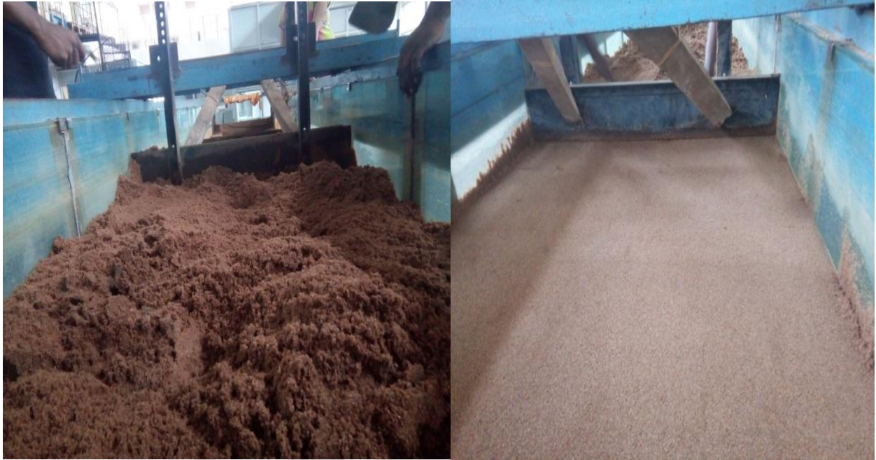
Figure 2.17: Steel frame for preparing flat non-uniform sand bed channel in the flume
