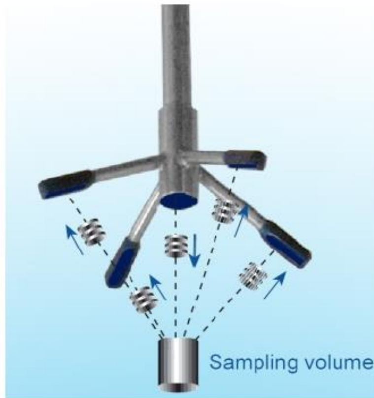
Figure 2.14: ADV and the remote sampling volume (Image source: Vectrino user guide)
