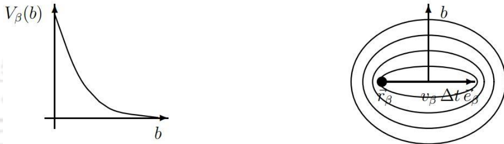
Figure 2.10. (a) Decrease of repulsive interaction potential V_{\beta}(b) with b , (b) Elliptical equipotential lines of V_{\beta} for different values of b (Source: Helbing, 1998)
