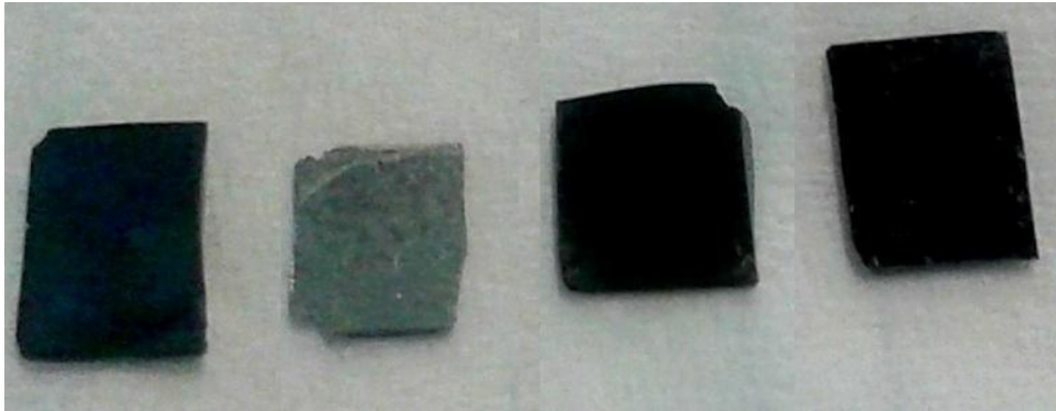
Fig. 7.3 From left porous Si substrate, Ni/Si, CNT/Ni/Si and CNT/Ni/CNT/Ni/Si films
