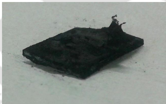
Fig. 7.2 Poor adhesion of CNT/Ni/CNT film
