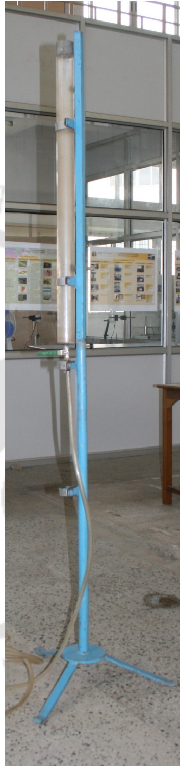
Fig. A.2. (a) Submerged jet apparatus with all the assembly, and (b) adjustable water head tank
