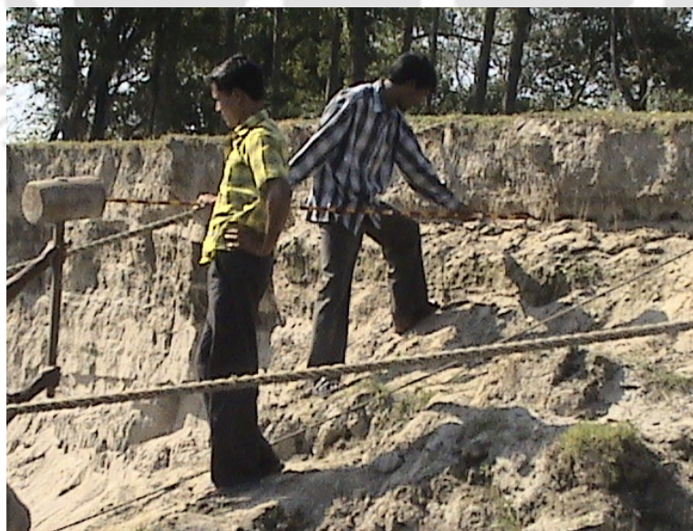
Fig. 3.17. Insertion of the erosion pins into the bank
