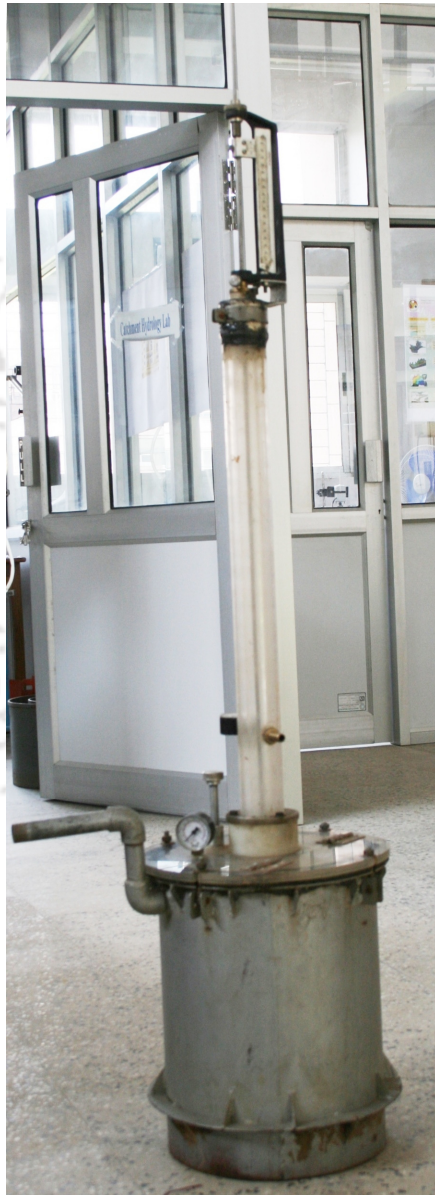
Fig. A.2. (a) Submerged jet apparatus with all the assembly, and (b) adjustable water head tank
