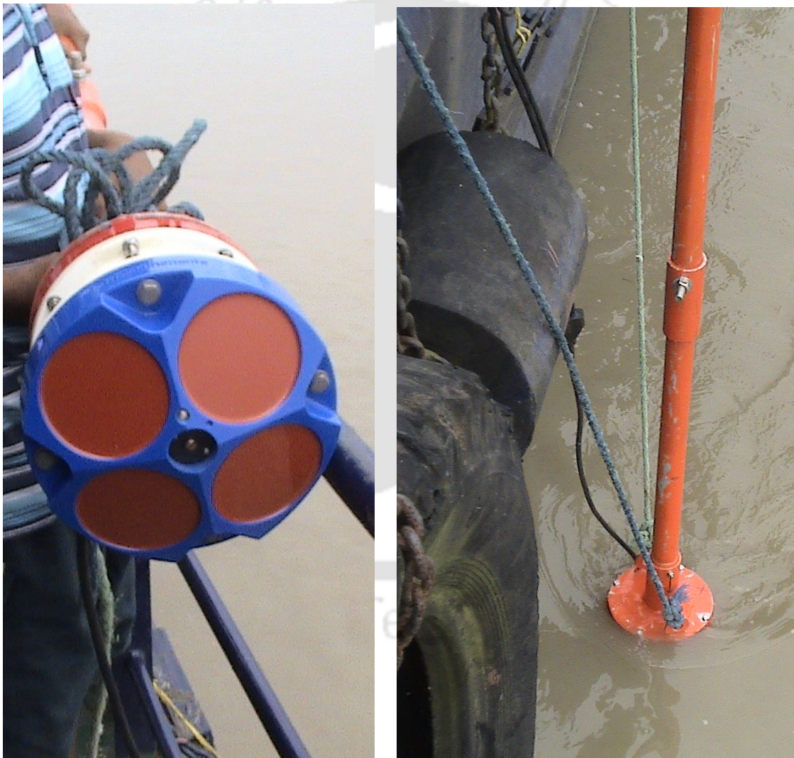
Fig.3.6. Photographs showing the ADCP instruments: (a) 4 transducers (b) installed in a survey vessel during data collection
