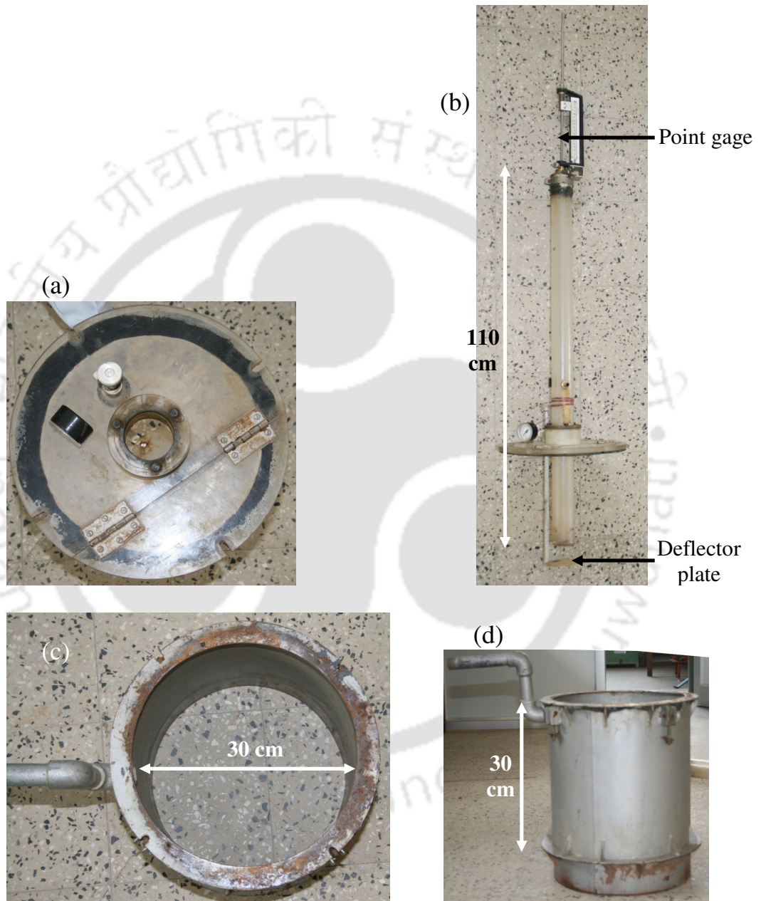
Fig. A.1. Submerged jet test apparatus: (a) Transparent top plate, (b) Jet tube with point gauge and deflector plate, (c) Top view of submergence tank (d) Side view of submergence tank
