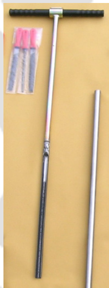
Fig. C.2. Sets of augers (Source: delta-T)
