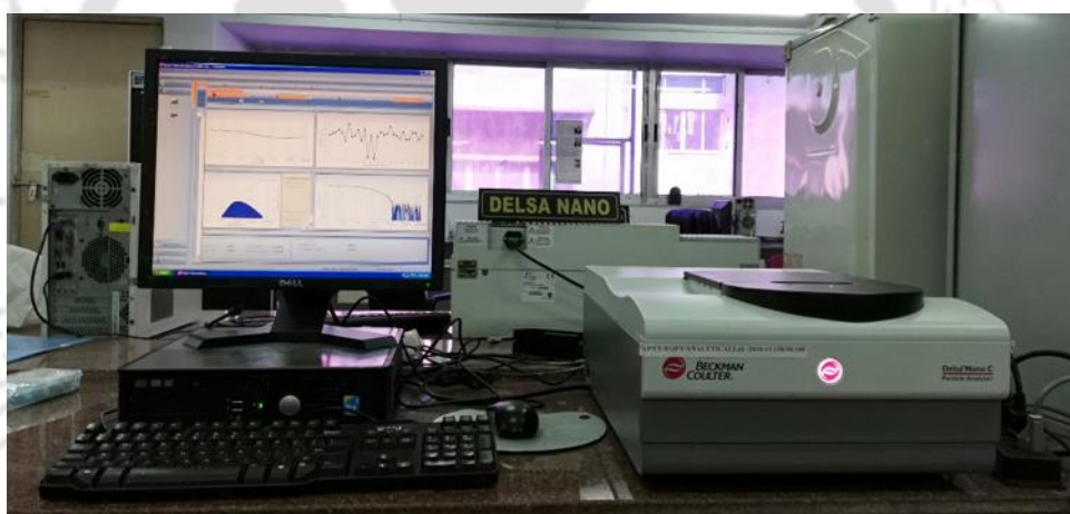
Figure 2.4. The equipment used for measuring the droplet size distribution and zeta potential.
