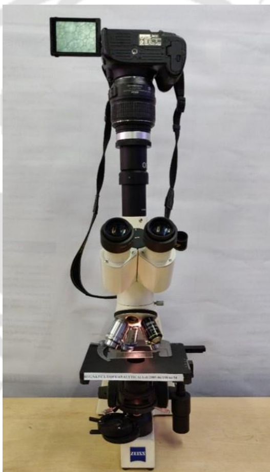
Figure 2.3. Experimental setup for taking photographs of foams using the microscope.
