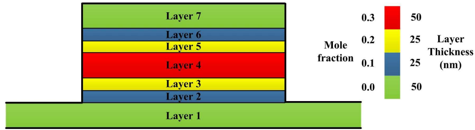
Fig. 6.1: Graded rib structure. The grading is along the x-axis with each layer doped P and N to form the PN phase shifter shown in Fig. 2.4. Layer 1 being relatively long and supported by the BOX and silicon substrate is unstrained while layers 2, 3, and 4 experiences biaxial compressive strain and layers 5, 6, and 7 biaxial tensile strain.
