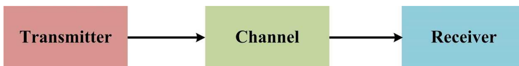
Fig. 2.1: Block diagram of a communication system.
