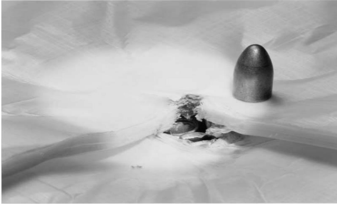
Figure 2-3 Penetration due to 9 mm Parabellum bullet in a soft ballistic package (Jacobs & Dingenen, 2001)
