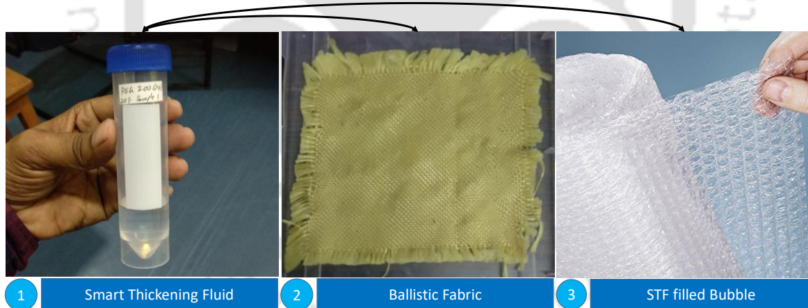
Figure 1-6 Basic constituent of liquid ballistic armour (1) Shear Thickening Fluid, (2) Ballistic Fabric, and (3) Schematic of STF filled Bubbles (Challenge, 2020).
