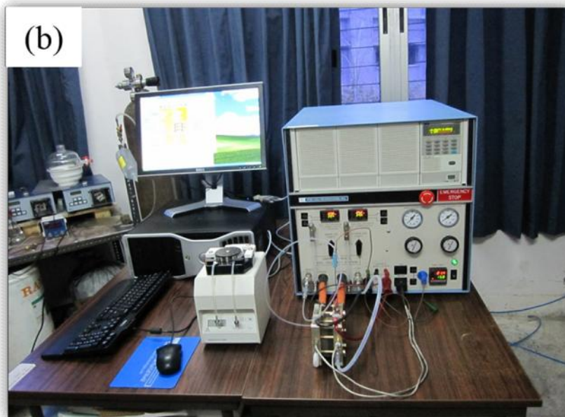
Figure 6.3: (a) Schematic of PEMFC testing station, and (b) snapshot of the PEMFC test station
