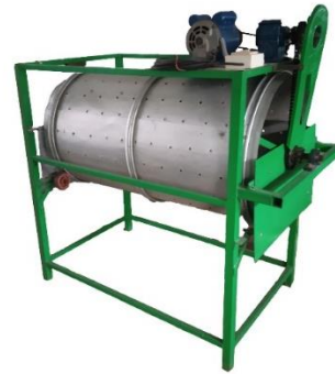
Figure 3.6: Final prototype of the washing machine.
