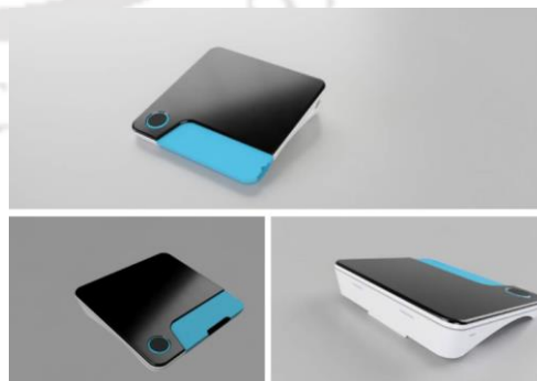
Figure N.16: CAD rendering of the finalized PoCT device concept. CAD models were developed for understanding the form, manufacturing and usability of
