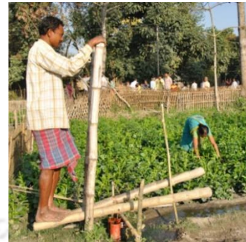
Figure 2.11: A man using the IDE Treadle Pump with Bamboo foot pedals. Image source: engineering4change.org [57]
