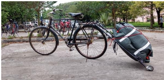
Figure N.43: First prototype of the product concept designed with a bag for bundling and transporting wet clothes.
