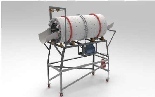
Figure N.31: CAD model of the first iteration of the ginger turmeric washing machine. CAD was used for detailing the product embodiment, finalizing product architecture and analysing it using DFM and DFMEA methods.
