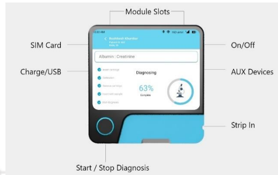
Figure N.18: The user interface and details of the concept. The Black part of the device is the computational module and the blue part is the swappable module for conducting various diagnostic tests using paper strips.
