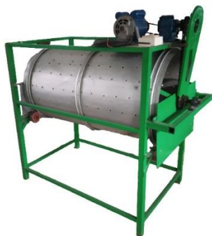
Figure N.33: Final prototype of the washing machine. The prototype was developed in collaboration with a grassroots innovator. Frugal mindset of the innovator enabled significant reduction of cost.
