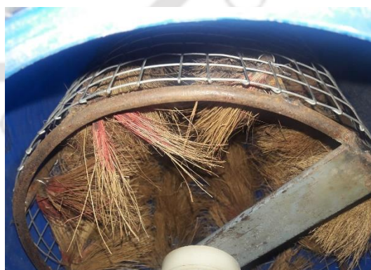
Figure N.28: The internal view of the 'jugaad' prototype. Coir brushes were used to create a way to dislodge dirt from the produce.
