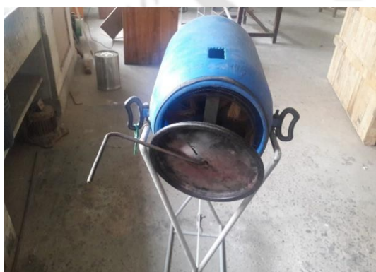
Figure N.27: A preliminary 'jugaad' prototype for the ginger turmeric washing machine. The team used readily available parts and components to create a prototype that enabled testing of the working principle.
