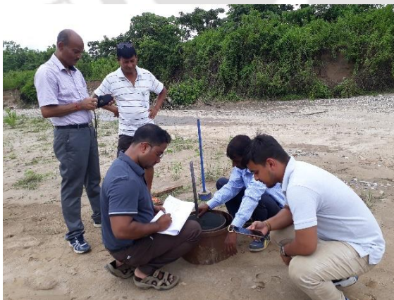
Figure 6.12 (c) Double ring infiltrometer test
