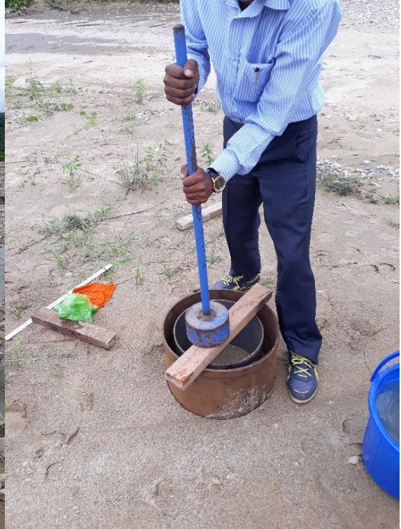
Figure 6.12 (b) Installation of double ring infiltrometer
