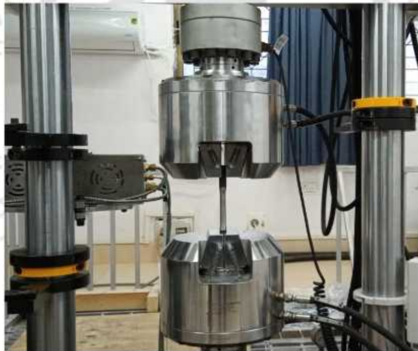
Fig.3.3 Test set up for coupon test
