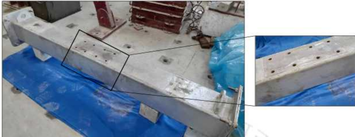
Fig. 5.6 Visual observation on panel zone and CFT column
