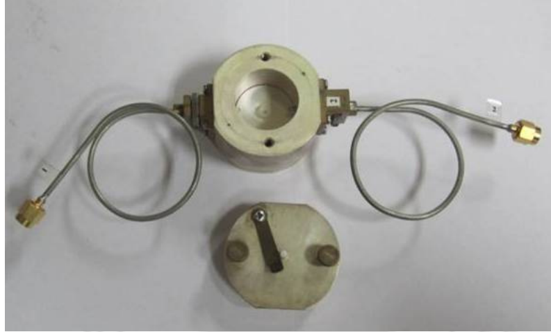
Figure 2.5: QWED Krupka resonator cavity used to measure the quality factor and dielectric constant.
