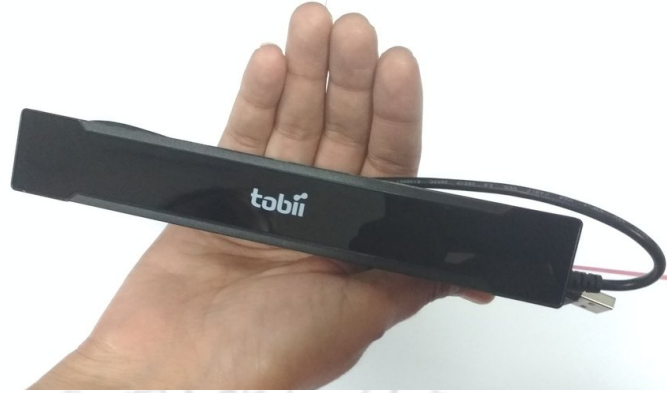
Figure 2.3: A prototype PCCR eye-tracker, Tobii X2-60
