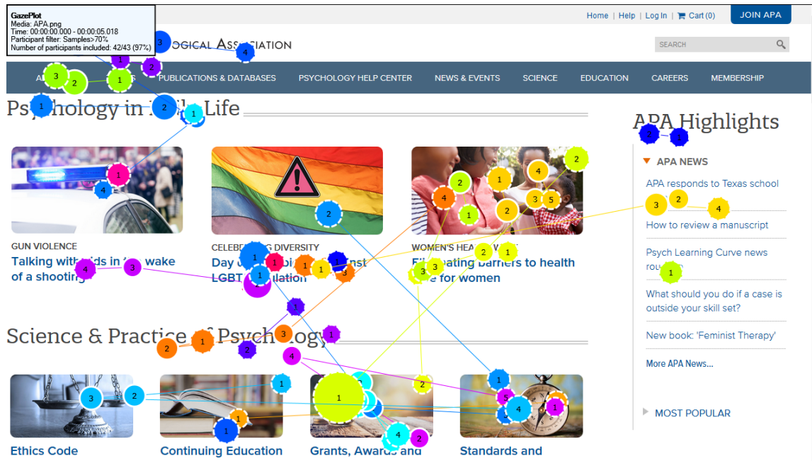
Figure 2.5: Example users' scanpaths on a webpage: Each bubble is a fixation with the inscribed number (fixation index) indicating the ordinal number of the fixation in a scanpath. Each user's scanpath is indicated with a different color.
