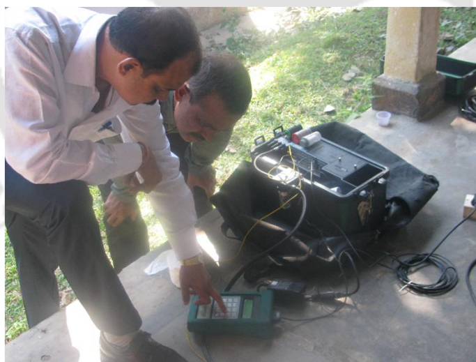
Figure 3.18 Exhaust gas analyzer and emission monitor
