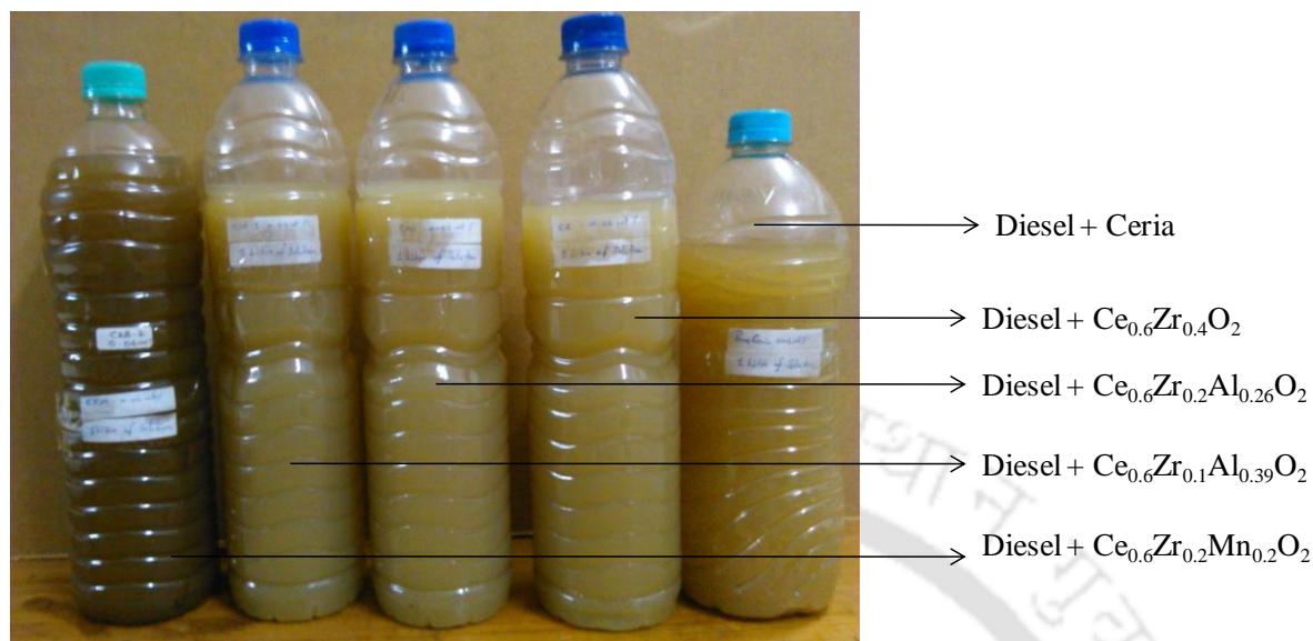
Figure 3.5 Different samples prepared using tip sonicator
