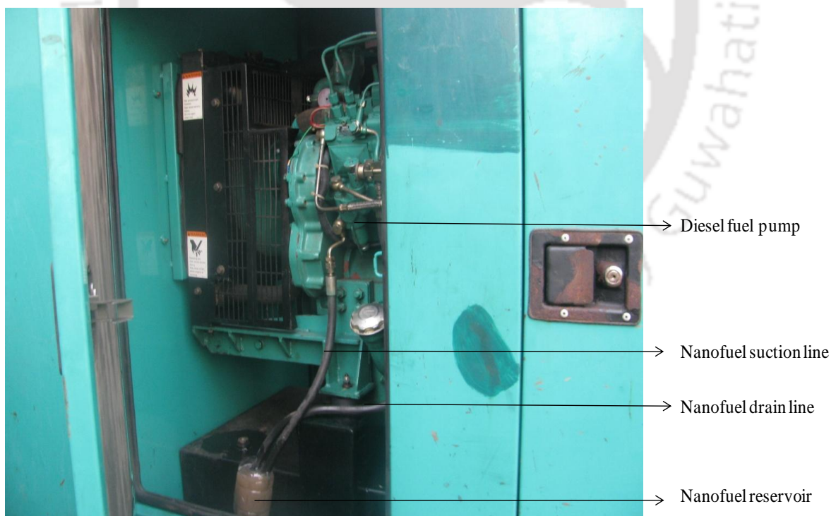
Figure 3.19 Suction and drained nanofuel line in the nanofuel reservoir
