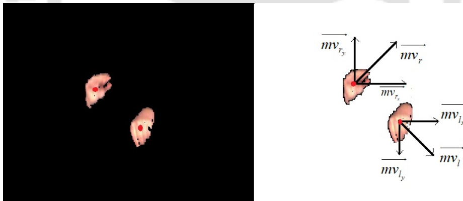
FIGURE 5.13: Finding movement of the hands (a) Centroids of the hands (b) Motion vector (mv) components for left and right hands.
