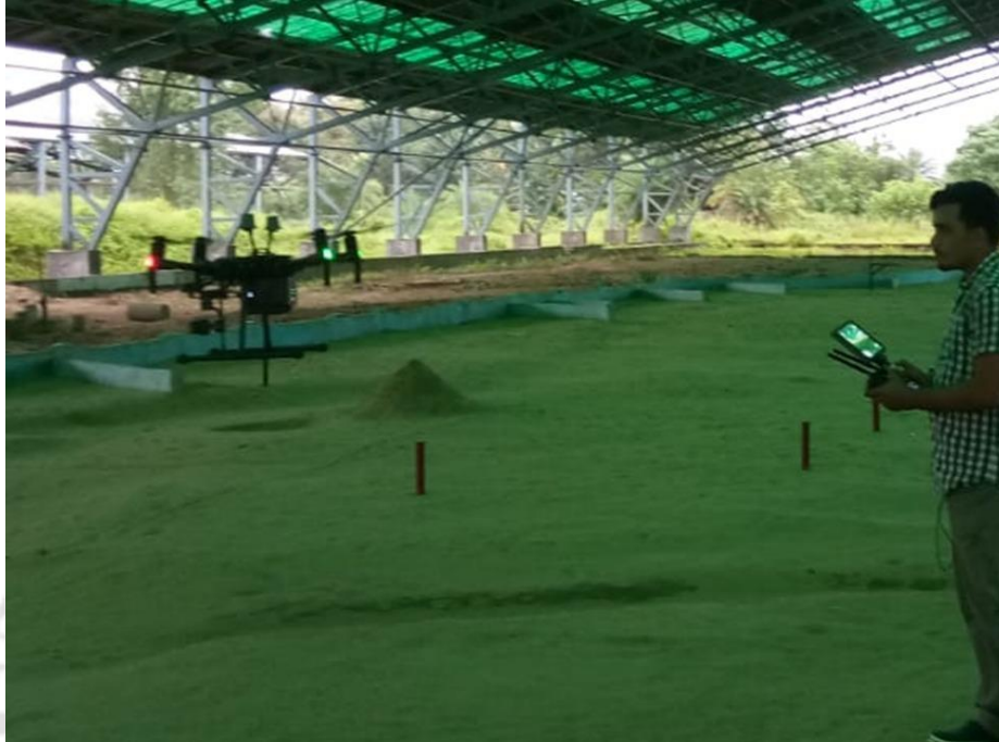
Figure 6.17 A photo during use of UAV to generate Digital Surface Models (DSMs) of model bed
