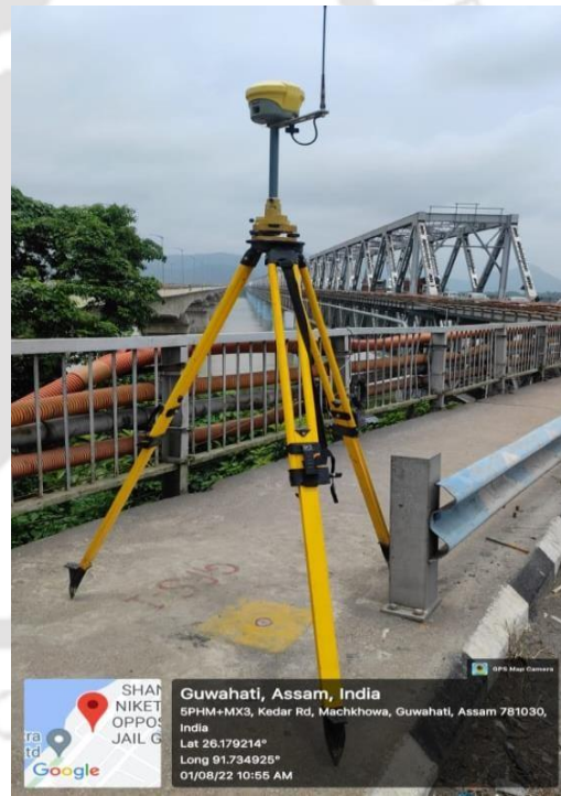
Figure 4.2 Photographs taken during bathymetry survey near Guwahati
