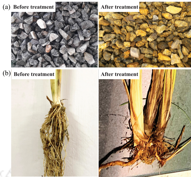
Fig. 3.9 Photographic image of (a) ferric hydroxide coating on gravel and (b) iron plaque formations on the roots after treatment in HSSF-CW (A).
