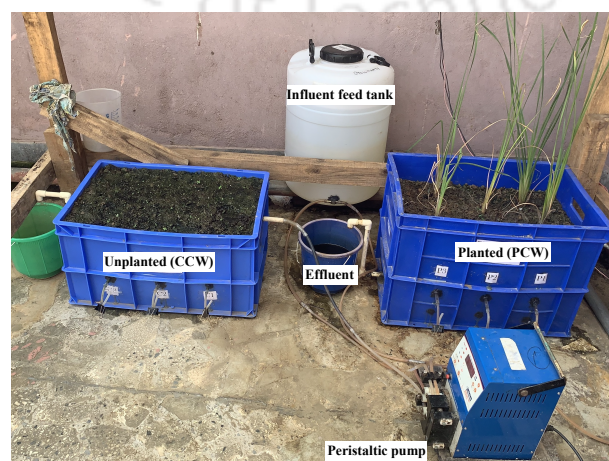
Fig. 4.3 Photographic image of CCW and PCW microcosms.
