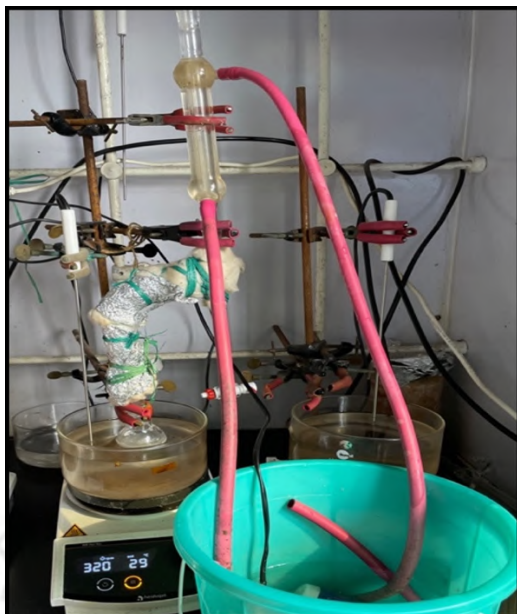
Figure 2.5 Dean-Stark apparatus used for determination of moisture content.
