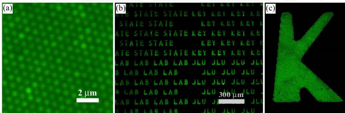
Figure 2.20: Polymer brush patterns mediated DNA sensing system. (a) Fluorescence image of the DNA nano-cone arrays with the period of 620 nm after binding the FITC-conjugate complementary oligonucleotide; (b) fluorescence image of hierarchical DNA patterns after binding FITC-conjugate complementary oligonucleotide. (c) The enlarged fluorescence photograph of the DNA pattern in image. [37]
