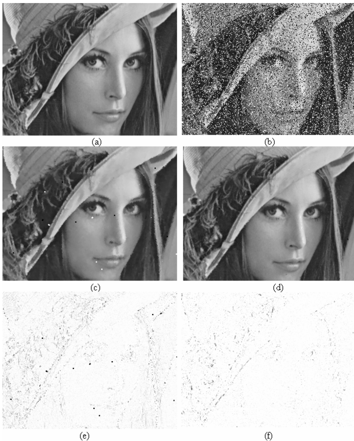
Figure 5.8a Outputs of various filters: (a) original Lena image (face portion), (b) the image with 20% fixed-valued impulse noise, (c) and (d) the outputs of the SM filter and 2-NCLPF ROM , (e) and (f) the magnitudes of differences between the original image and (c) and (d) respectively.
