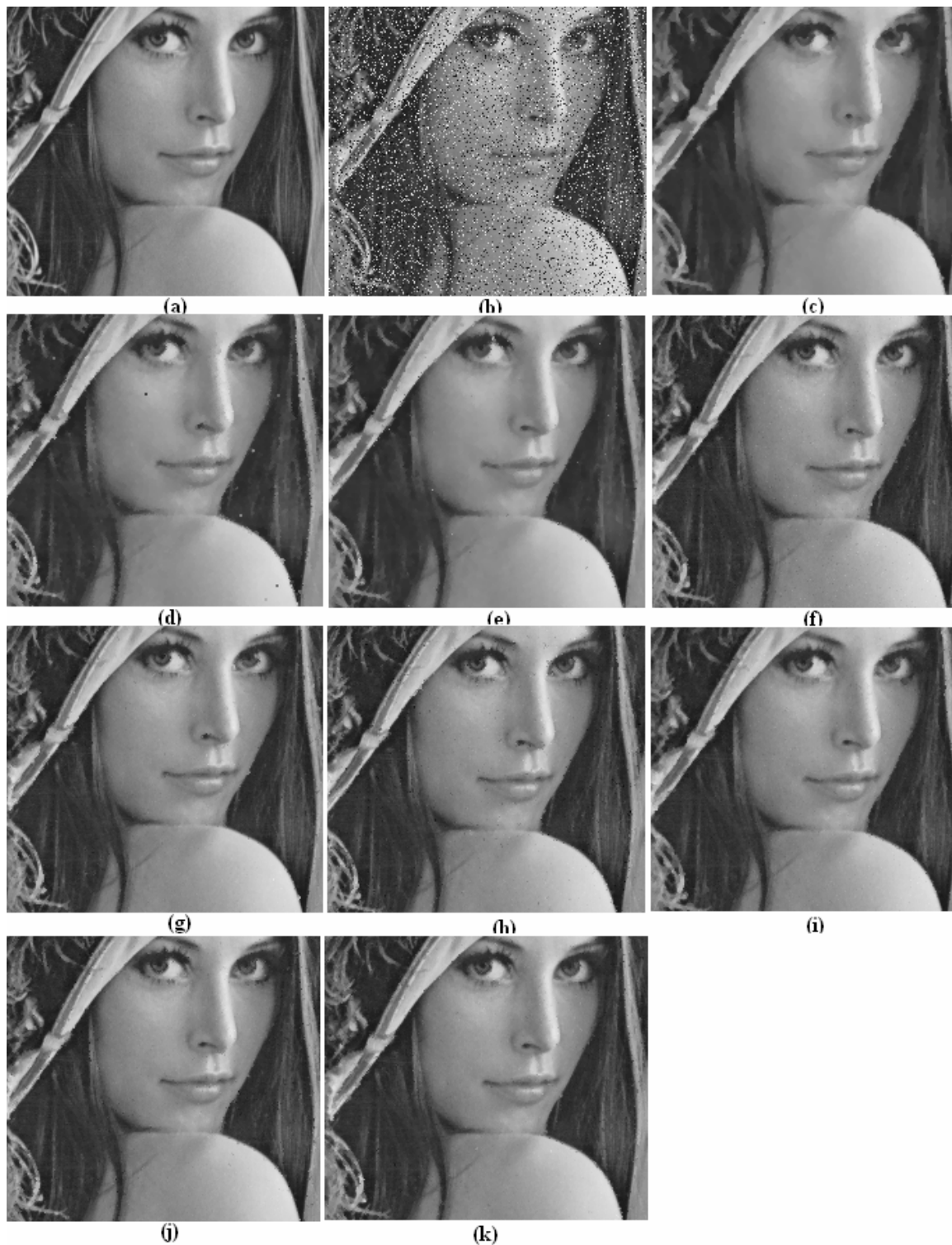
Figure 3.7 Outputs of various filters on the Lena image: (a) original image (part), (b) Image corrupted with 20% random-valued impulse noise, (c), (d), (e), (f), (g), (h), (i) (j) and (k) - outputs of the SM, CWM, RCM, TSM, SD-ROM, Chen and Wu, RCT-I, -II and -III filters.
