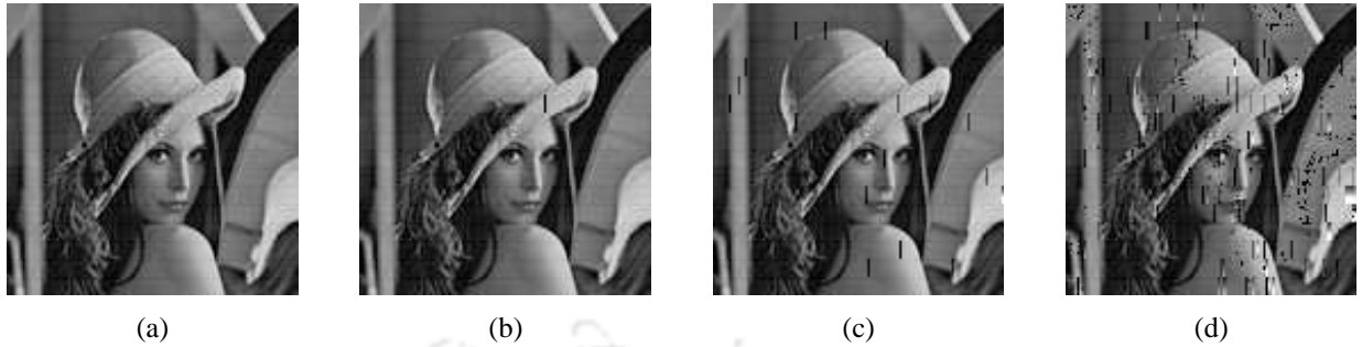
Figure 5.12: Image processing results using (32 \times 32) -bit ApproxMAC with: (a) k = 48 ; (b) k = 40 ; (c) k = 32 ; and (d) k = 24 .
