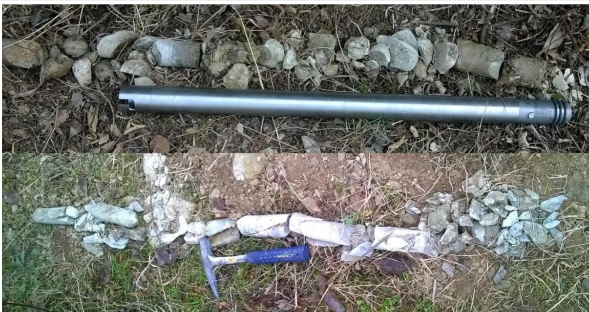
Photograph 5.4. Rock Cores collected during the drilling exercise at selected hydrological response unit (HRU).
