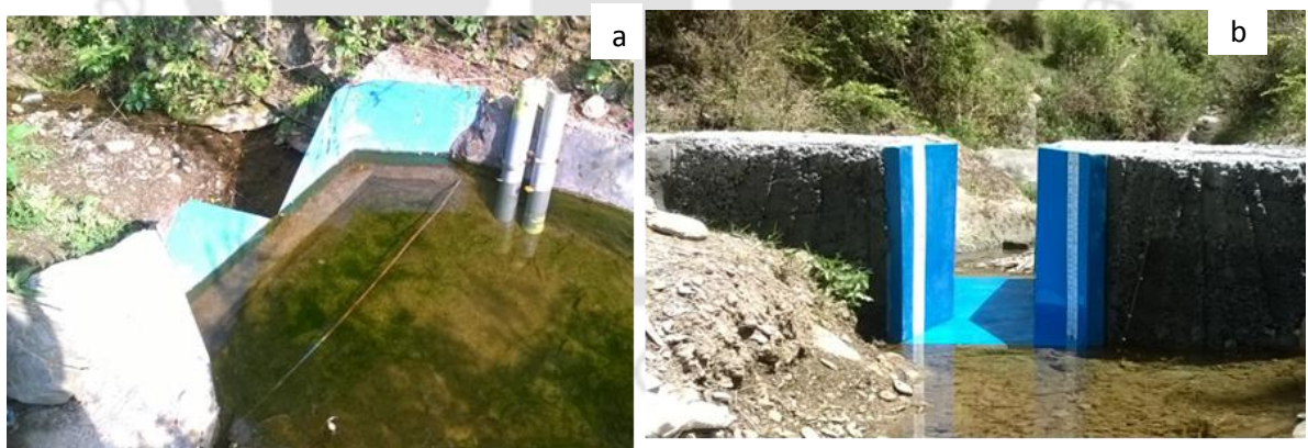
Photograph 2.1: Right angle V-notch (a) at the outlet of Bhimlitali catchment and cutthroat flume (b) at the outlet of the Dugar Gad headwater catchment.
