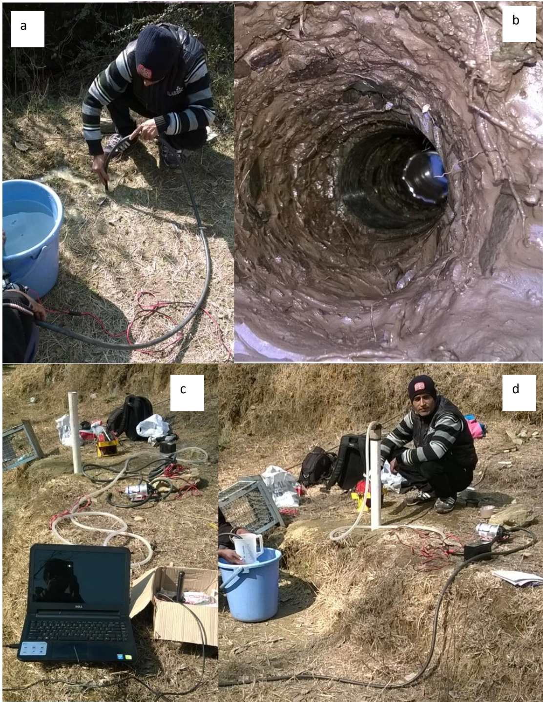
Photograph 5.2: Borewell development through ejection of clean water (a), a cleaned shallow borewell with DWL of less than 150 cm in central narrow riparian valley (b), setup of equipments for pump test and slug test experimentation in shallow borewell 1 in the study site (c& d).
