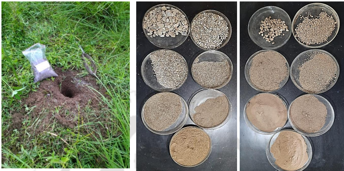
Photograph 8.2: Soil sample collection from different land cover areas and separation of soil particles through electromagnetic sieve analysis method.
