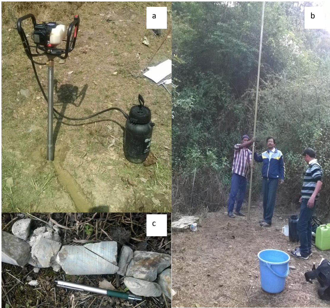
Photograph 5.3. ShawBackback Drill with engine pressurized water supply and drill rod (a), close-up of rock core with fractured quartzite (b), deepest borewell (BW 6) of 6 m in the hill slope of the micro-catchment.
