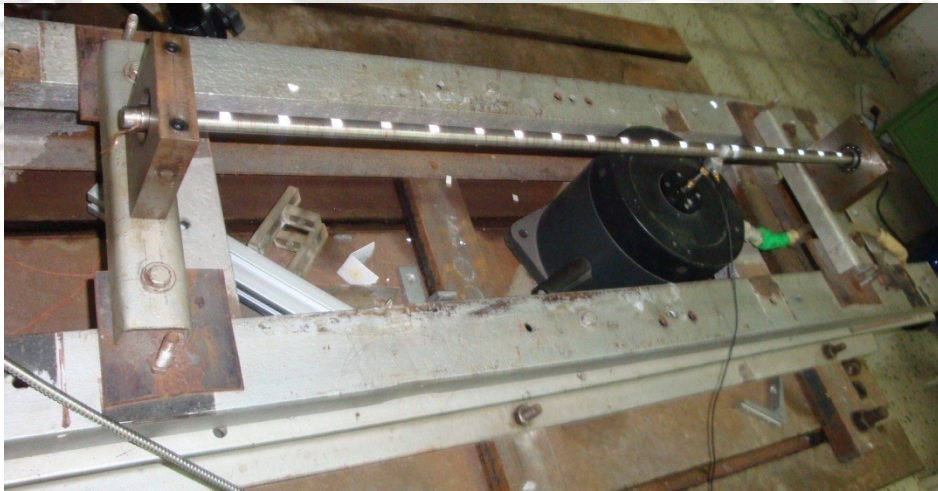
Figure 6.1: The test rig for the experimental crack detection.
