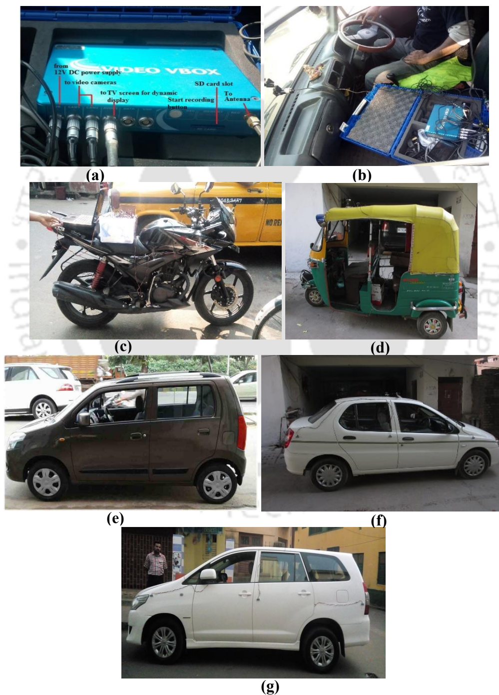
Figure 3-2 (a) Details of Video VBOX data recording Unit (b) Video VBOX installed in a car (c) Motorized two-wheeler (2W) (d) Motorized three-wheeler (3W) (e) H-Back Car (f) Sedan Car (g) SUV car
