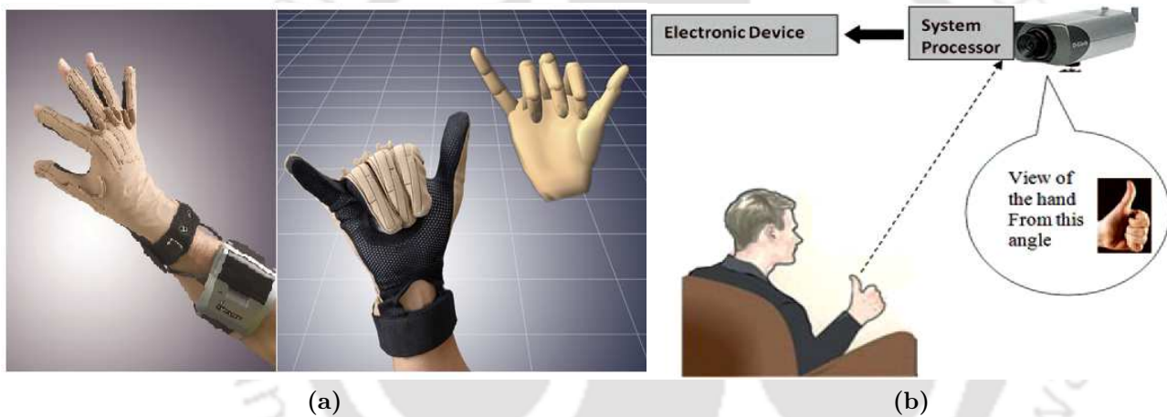
Figure 1.3: Human-Computer Interaction using: (a) CyberGlove-II, (b) Vision-based system [1].
