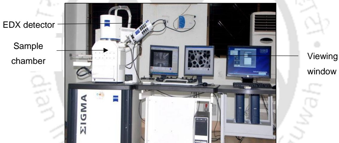
Figure 3.10 Field Emission Scanning Electron Microscope (Make: Zeiss, Model: Sigma)
