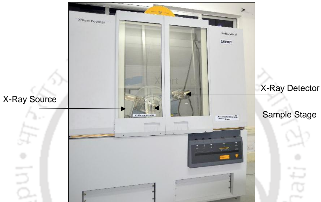
Figure 3.8 X-ray Diffractometer (Make: PANalytical, Model: X'Pert powder)
