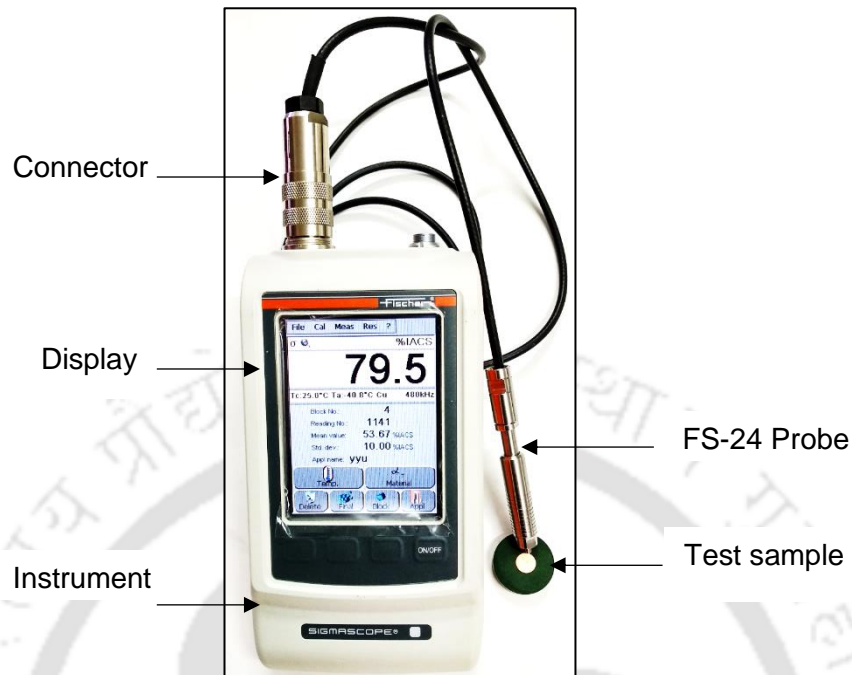
Figure 3.16 Electrical conductivity instrument - Sigmascope SMP350
