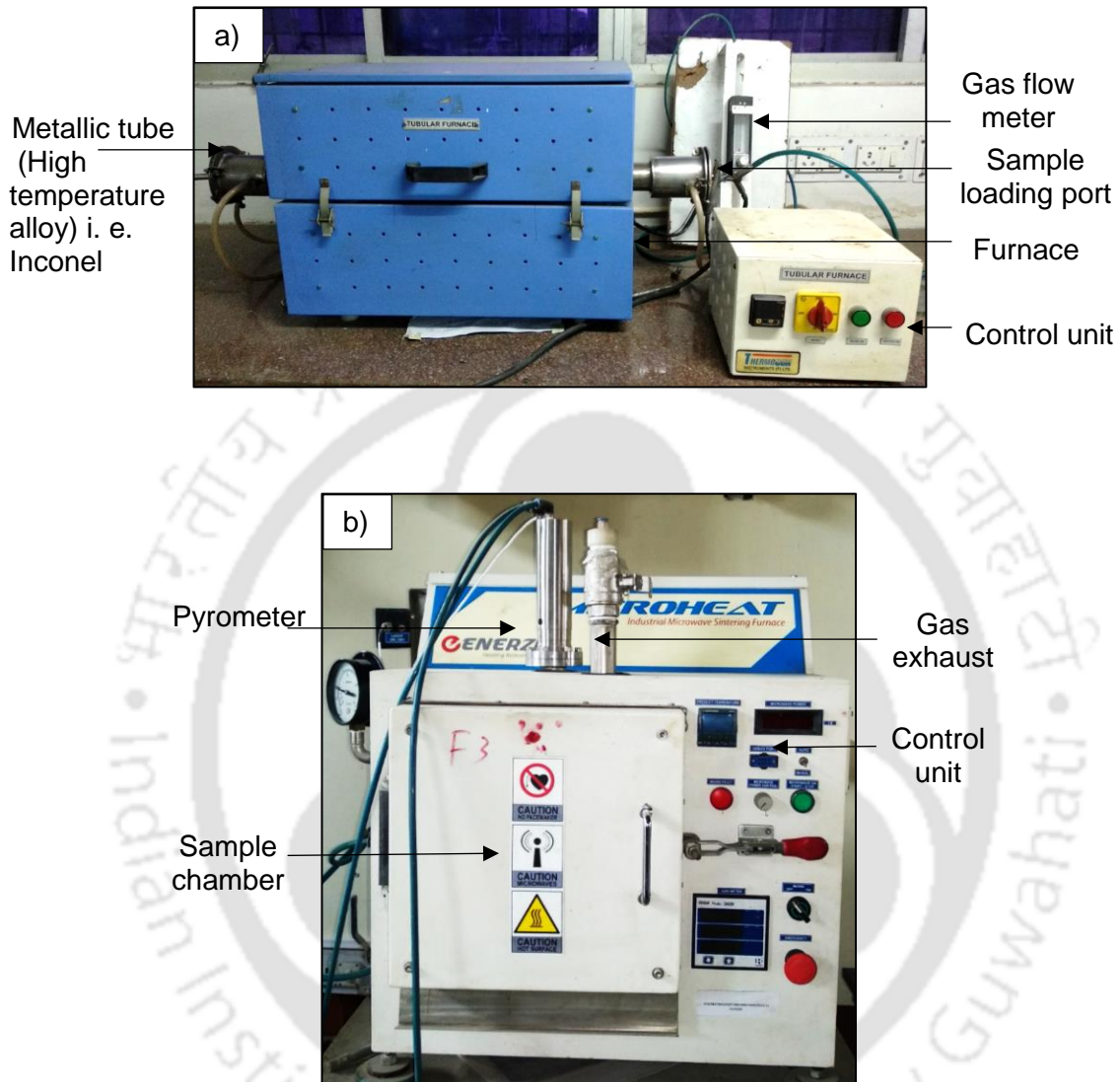
Figure 3.5 a) Conventional tubular sintering furnace and b) Microwave sintering furnace
